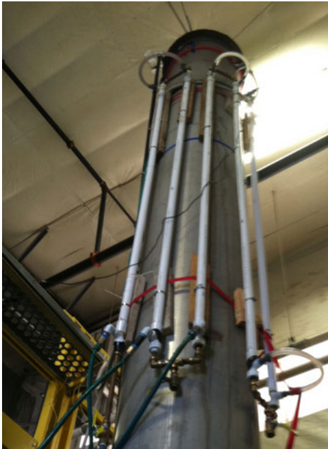
Heat exchanger attached to 1600L
